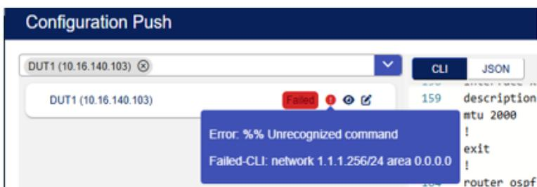
Note: HINT: You can use the CLI on a device to help you construct and format a payload using the `show json running-config` command.
