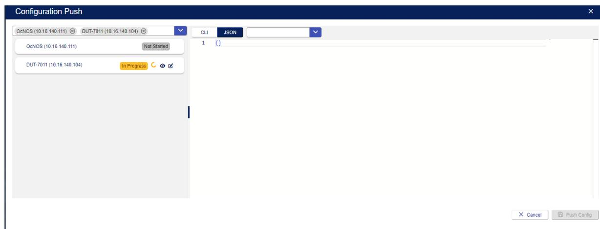
The code editor implements IntelliSense and validation including basic syntax checking and coloring and the intended payload consists of NETCONF YANG model segments in JSON format.
